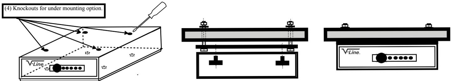
1. Remove the drawer completely out of the case's outer shell by releasing the black plastic slider tabs on the inside of the sliders.
